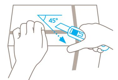
For best results, cut plastic strapping band **diagonally** (at a 45° angle).
