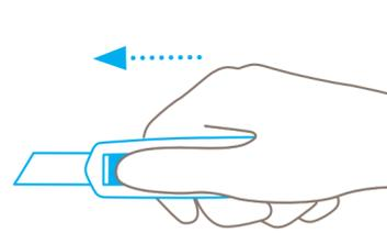
Use the slider to **engage the blade** for cutting.
