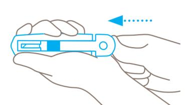
Make sure you position the blade **exactly over the locating lugs**, close the blade holder upwards. **Attention:** Never hold your hand in front of the blade exit!
