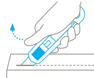
Always remove your **thumb from the slider** to ensure automatic blade retraction.
