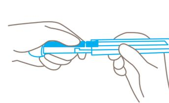
When the slider and blade leave the handle, position your **index finger under the blue blade holder** to hold it tight.
