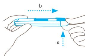
Press the blade change button **pushing up from below** and remove the plastic insert from the rear of the handle.
